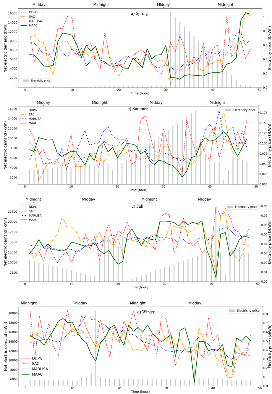
Fig. 6. Net electricity demand curves of different RL-based controllers in response to the electricity price during 48-hour periods in seasons of (a) spring, (b) summer, (c) fall, and (d) winter.
